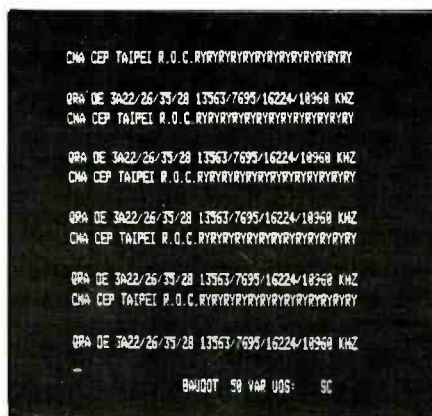
A marker slip from an RTTY station in Taipei, Republic of Free China. This station has been monitored on 7695, 10960, 13563, and 16224 kHz.
